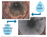
Comparison of corrosion inside pipes
