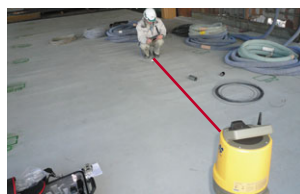
3D-MAPS laser radiation *Illustration of laser beam on the photograph.
