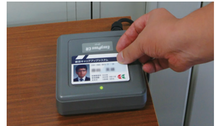
Card reader of Construction Career Up System
