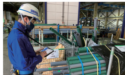
Inspection of Piping Parts Fabricated at the Plant
